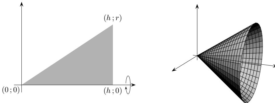
$$\begin{aligned} \pi \int_0^h \left(\frac{r}{h}x\right)^2 dx &= \pi \int_0^h \frac{r^2}{h^2} x^2 dx = \pi \left( \frac{r^2}{h^2} \cdot \frac{1}{3} x^3 \Big|_0^h \right) = \\ \pi \left( \left(\frac{r^2}{h^2} \cdot \frac{1}{3} h^3\right) - \left(\frac{r^2}{h^2} \cdot \frac{1}{3} \cdot 0^3\right) \right) &= \pi \cdot \frac{r^2}{h^2} \cdot \frac{1}{3} h^3 = \frac{1}{3} \pi r^2 h \end{aligned}$$
